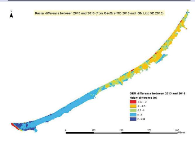
**Figure 38** Topographic Grid time analysis: subtraction of the elevation from one date to another to obtain erosion and accumulation for each pixel (BRGM)
