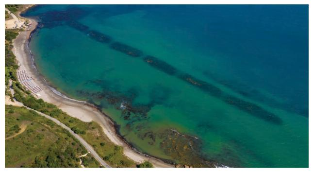
Figure 47 Submerged breakwaters)
