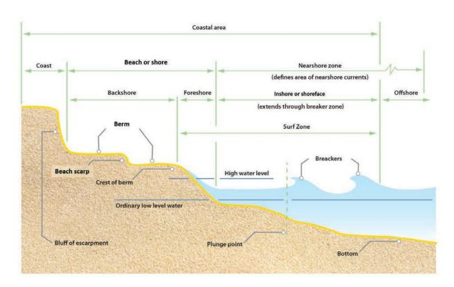
Figure 2. Terminology of a beach profile (as taken from Shore Protection Manual, 1984).
