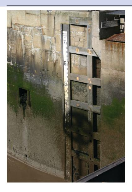
**Figure 35.** Tide monitoring: tide gauge
