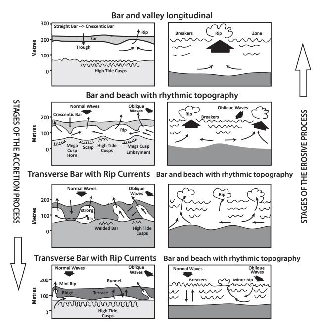
**Figure 14.** Plan view of the sequence of changes in the morphology of the beach and its submarine area in an accretion process (left graph) and in an erosive process (right graph) (Short, (1999), based on Short, (1979); Wright and Short, (1984); Sunamura
