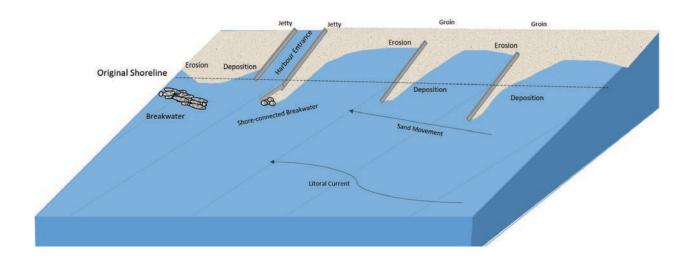
**Figure 19**: Interruption of longshore sediment transport caused by coastal structures, from https://anserosion.weebly.com/coastal-processes.html
