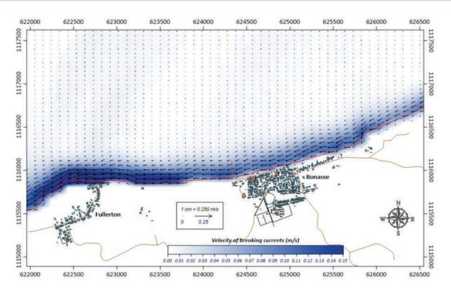
**Figure 42** Example of the output of a coastal circulation model used by Inversiones Gamma in its execution of the executive beach restoration project at Bonasse Beach in Cedros Bay, Trinidad and Tobago.
