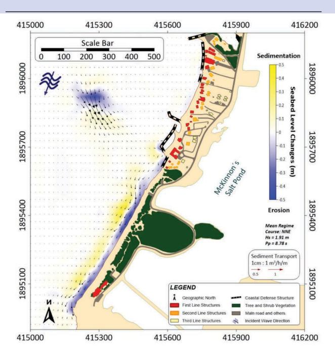
**Figure 43** Example of sediment transport and morphology change modelling carried out by Inversiones Gamma for the executive beach restoration project at Runaway Bay Beach in Antiagua and Barbuda. Taken from the report by Morales Diaz et al. (2022).
