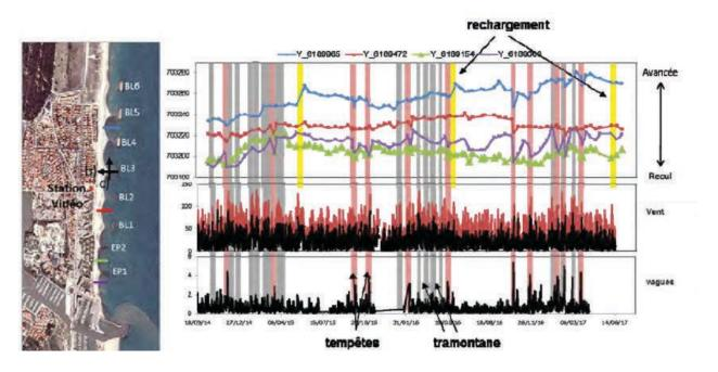
**Figure 39** Time series with superposition of coastline positions (colors related to profiles), wind and waves (top to bottom)
