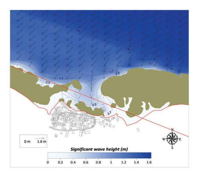
**Figure 41** Example of numerical wave modeling conducted by Inversiones Gamma in its execution of the executive beach restoration project at Bonasse Beach in Cedros Bay, Trinidad and Tobago. Shown are wave heights (shades of blue) and wave direction.
