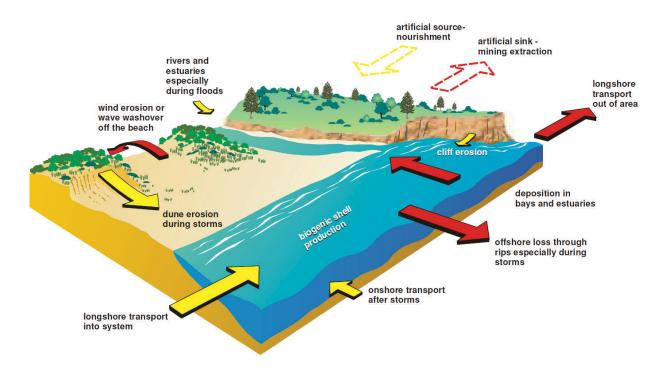
**Figure 17:** Some components of a sediment budget, taken from NSW Department of Land and Water Conservation 2001, Coastal Dune Management: A Manual of Coastal Dune Management and Rehabilitation Techniques, Coastal Unit, DLWC, Newcastle
