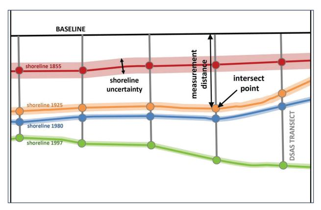
**Figure 36** DSAS generates transects that are cast perpendicular to the reference baseline at a user-specified spacing alongshore. DSAS measures the distance between the baseline and each shoreline intersection along a transect, and combines date information, and positional uncertainty for each shoreline
